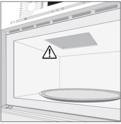
Do not remove the cover to the microwave outlet inside the oven.
